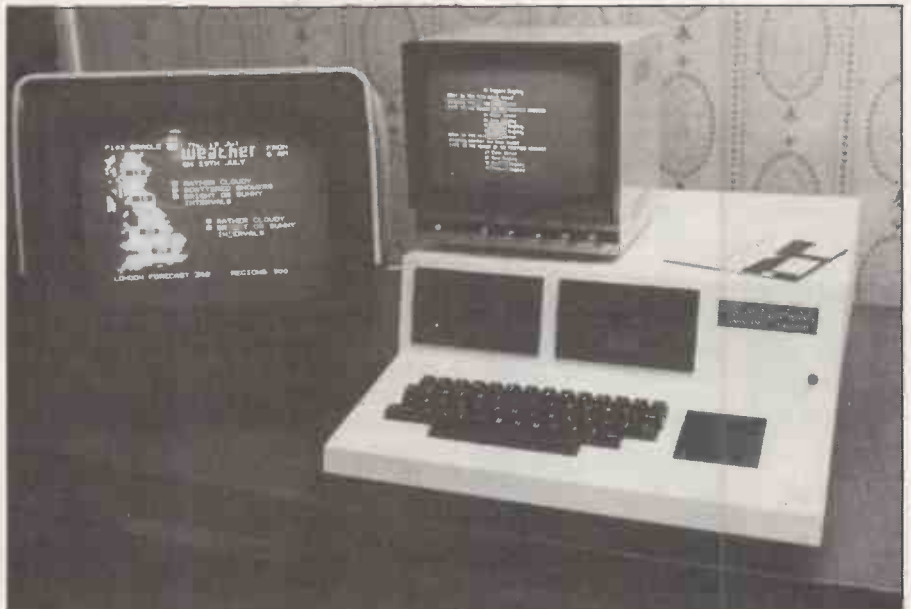
The Hi-Tech card interfaced to the Tuscan S-100 bus.
